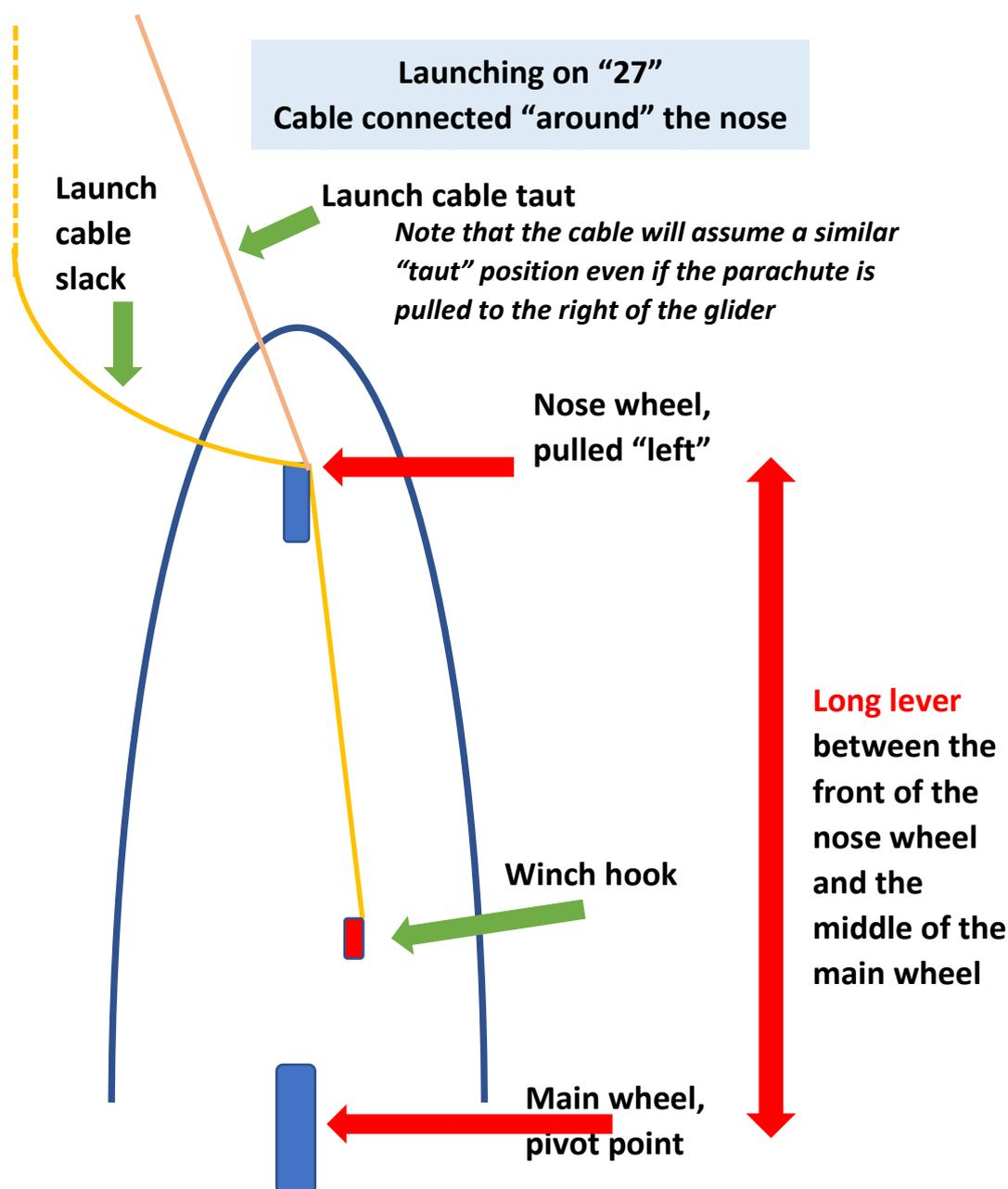
Note that **the lever-arm** pulling the nose left is from the front of the nose wheel to the middle of the main wheel, which **is several feet** (metres) long.
