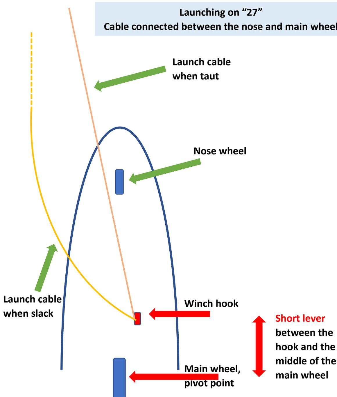
As should be evident, passing the cable between the wheels will significantly reduce (but not eliminate) the tendency for the Perkoz to swing-left on launch.
