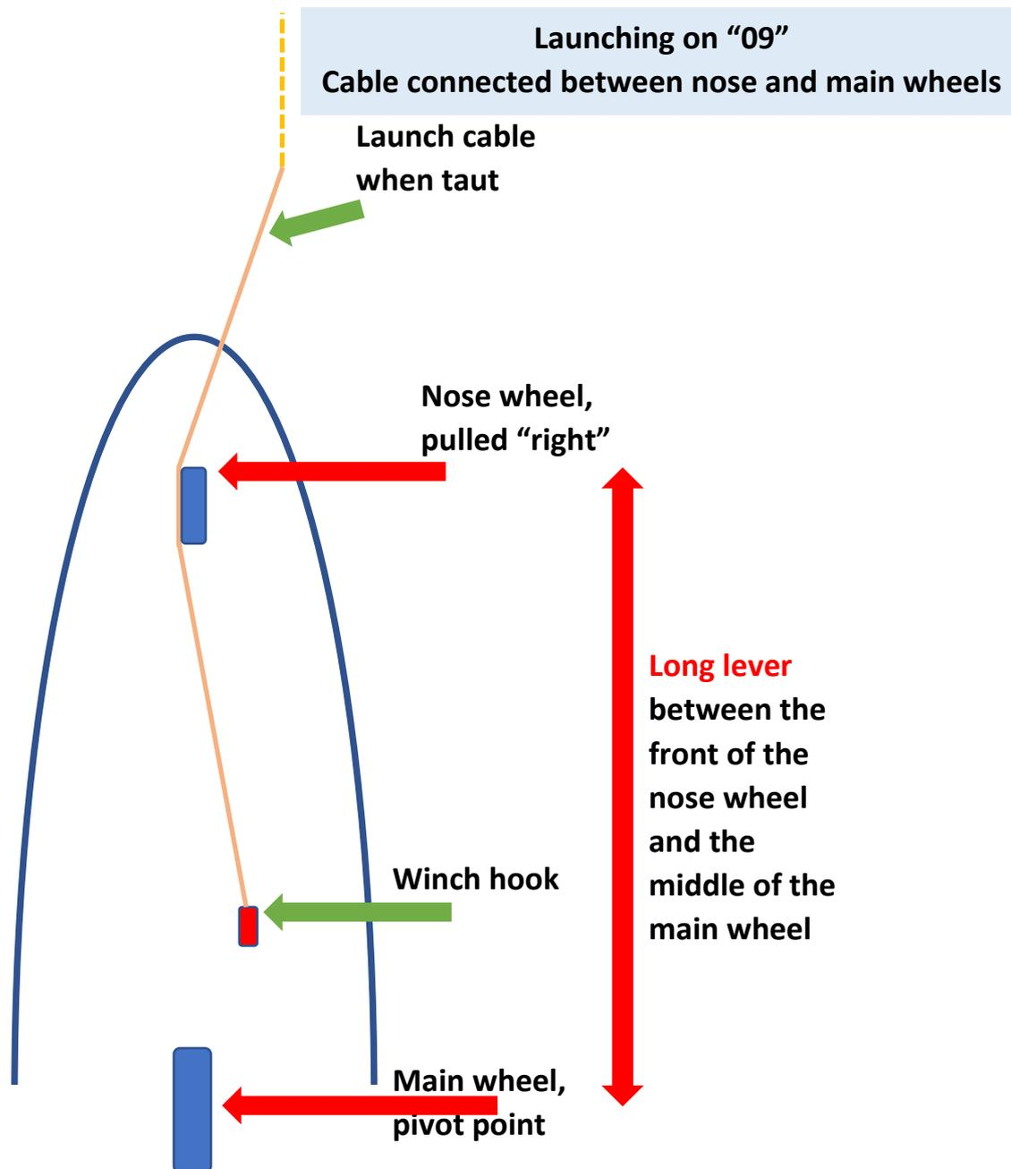
If the pilot does not lift the nose wheel quickly, then the cable will pull the nose to starboard (right), and that pull will be over a **long lever** arm and so it is likely to cause the Perkoz to swing right. So, in this situation, threading the cable between the wheels has caused an unnecessary control problem.
