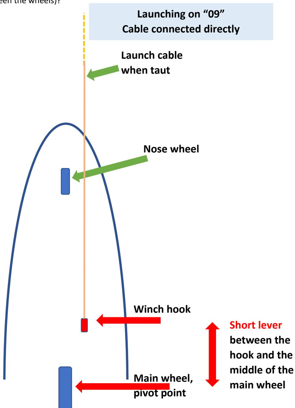
Here, when the cable pulls tight, it does not wrap around the nose wheel if it is connected "directly" to the hook. The **lever-arm is short**, and so there is a slight tendency to swing, caused by the offset hook position.
