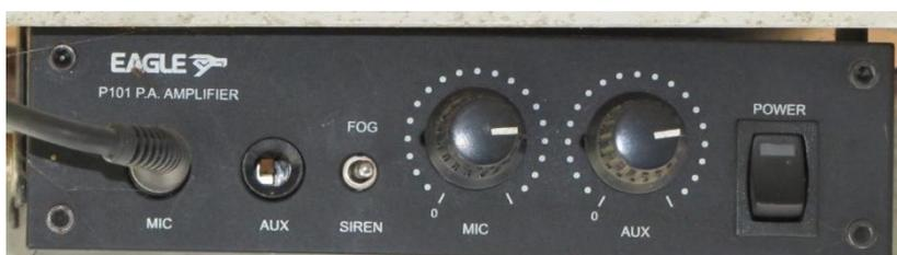
The PA system is not a radio but is located beside the radios on the overhead shelf. The microphone for this is located in a holder between the windows.
