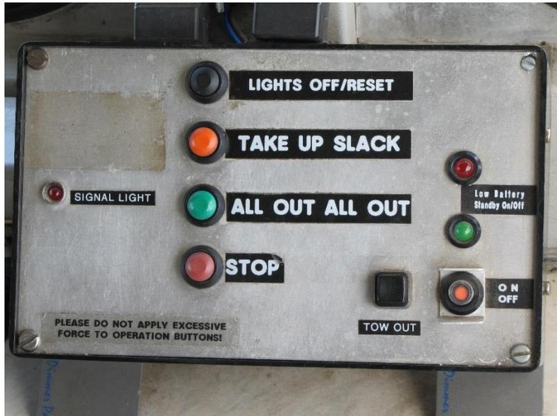
The launch point lights are controlled by a set of push-buttons at the launch point which cause the signal light to be off, on, or flash at an appropriate rate. The signal switch box makes a “beep” sound when the signal lamp is illuminated.
