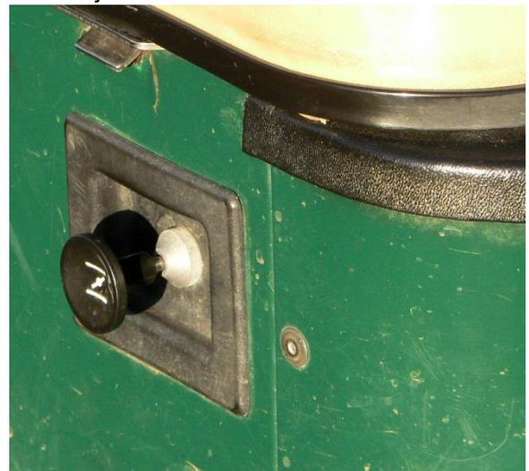
Always ensure that the path is clear before trying to start a buggy. It may require a relatively high engine rpm to keep it running (from cold) and the automatic clutch may engage the drive. There is a "neutral" position for the drive selector (located between the seats on the forward-facing panel); this is when the selector is vertical, although there is no positive stop for it in this position. If someone has parked the buggy facing toward something else then select
