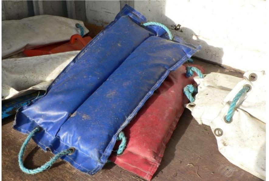
Take care not to put wing weights on fibreglass wing tips which might be crushed. Many gliders have a thin surface covering over a soft balsa wood (or similar) light filling material. Deforming the surface may permanently compress this material leaving a permanent distortion.
