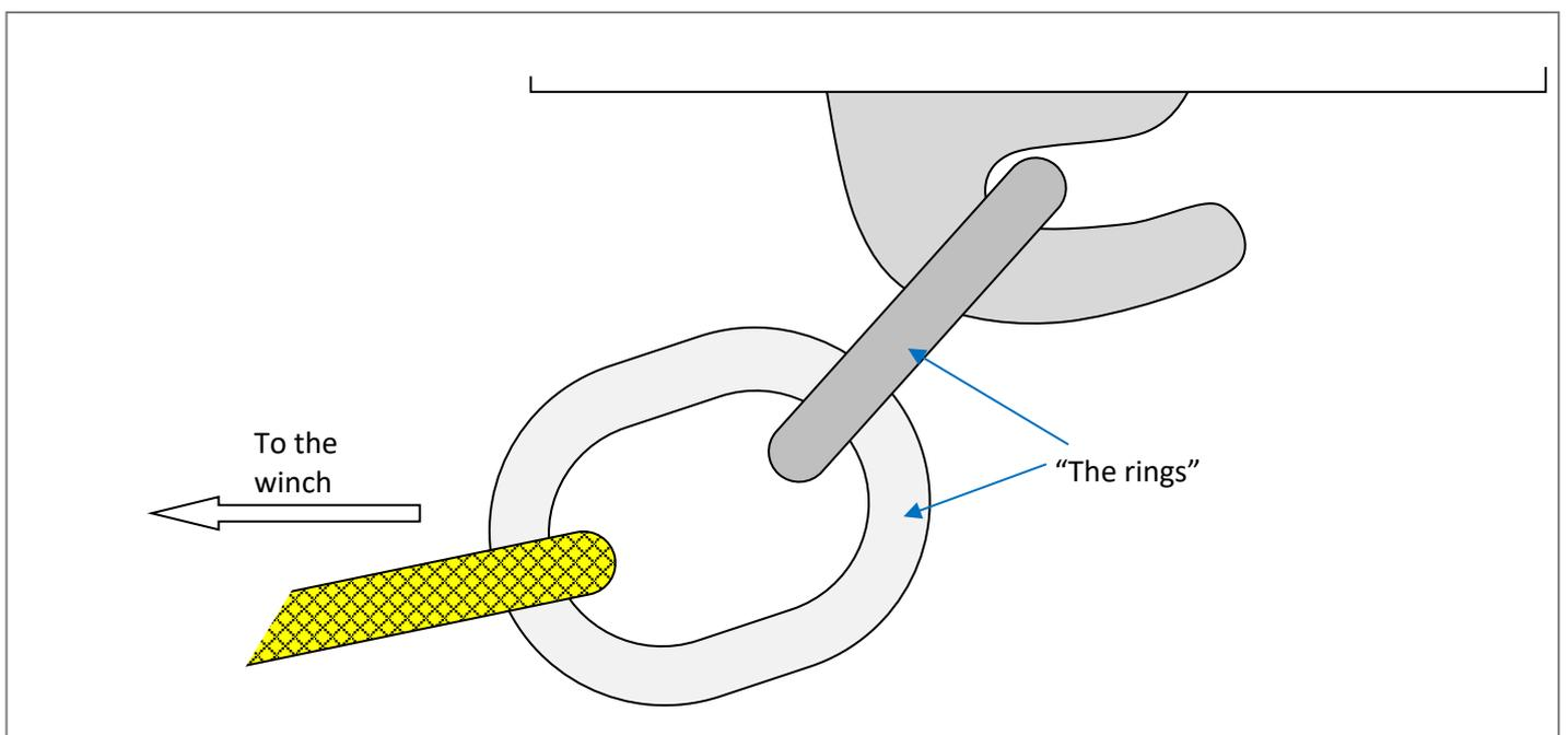
The hook itself engages with the ring to allow the glider to be pulled forwards and aloft. In most gliders it projects just below the bottom surface of the fuselage. It is encircled by the back-release ring and side plates which
