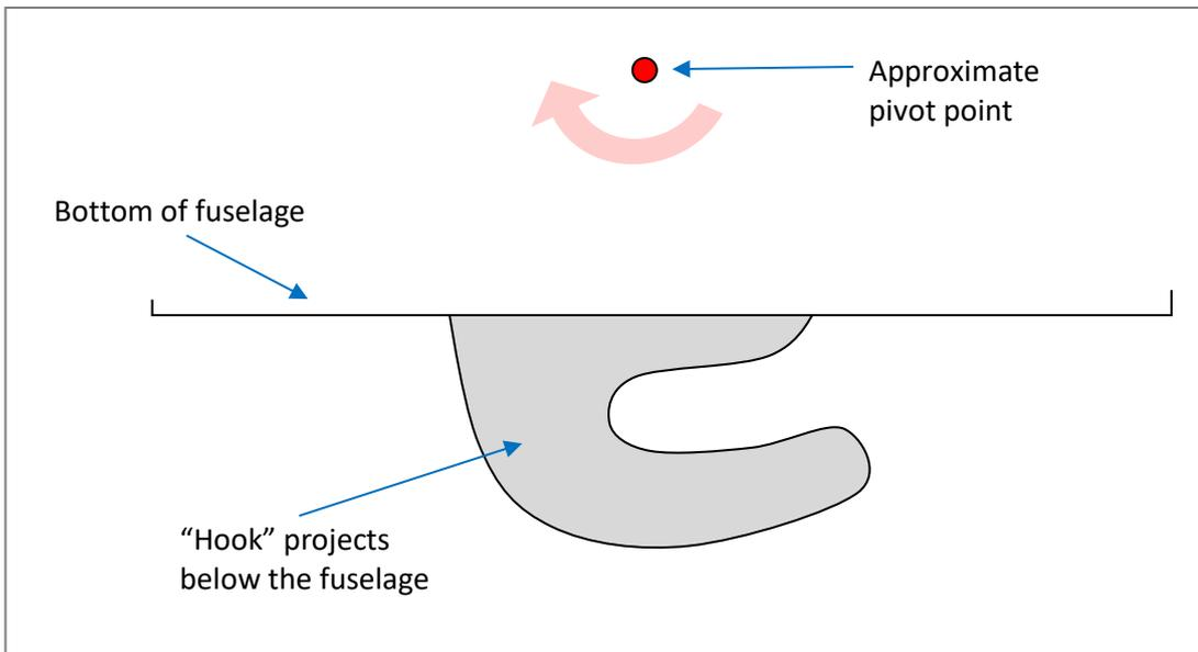
“The hook” is much more than just a hook. It incorporates the release mechanism operated by the pilot and a back-release mechanism that allows the ring to detach if it is not pulling the glider forwards.
