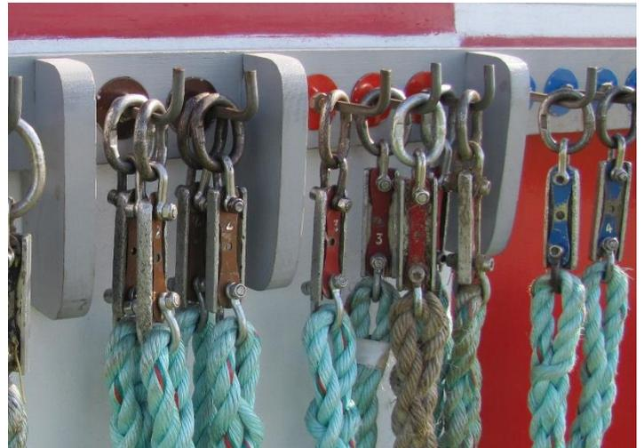
Weak links are normally stored on a rack on the outside of the launch vehicle. Please replace them there when not in use, this will prevent them from being lost, help us to keep them clean and available for use, and avoid them being damaged when run over by one of the vehicles
