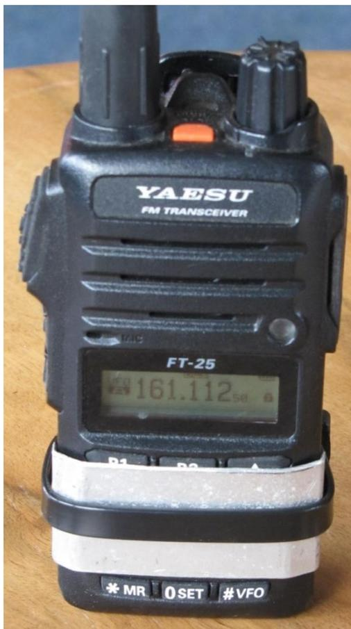
**On/Off** The push button at the bottom of the older radios turns them on and off. The newer (FT-25) radios have an **on/off – volume** rotary control on the top
