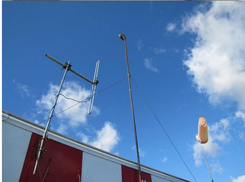
The light signals can only work if the light is pointing towards the winch. Whenever the winch or launch point cabin is moved it will be necessary to re-align the light so that it is clearly visible from the winch. This is usually done by using the radio and getting the winch driver to say when the “stop” signal is most visible while slackening the clamp and rotating the light appropriately.
