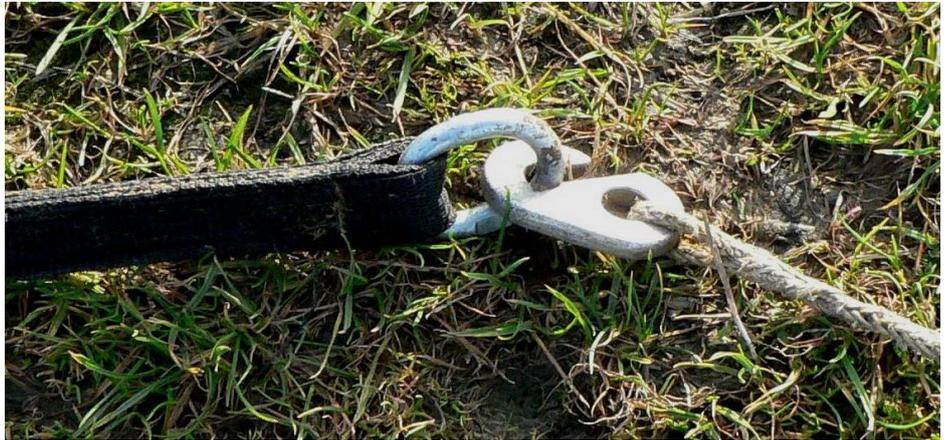
Be alert to the gap in the hook wearing. If it becomes enlarged then there could be failures or loss of equipment if it disengages inappropriately (for instance just after the glider has released).
