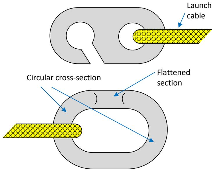
The hook is made from a flat plate with a slot machined to be just wide enough to slide over the flattened cross-section of the ring. The main hole in the hook is wider, so that the ring may be rotated to the “pulling” orientation (along the axis of the main oval) which prevents it from disengaging, because the circular cross-section of the majority of the ring is too big to slide through the jaws of the slot in the hook.
