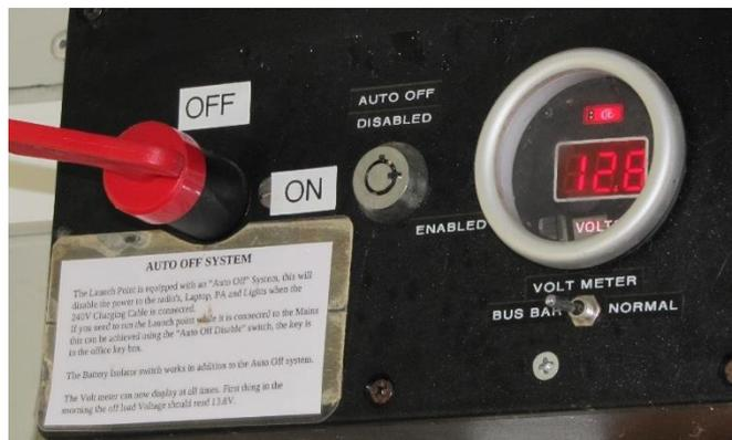
The main power switch in the launch point cabin is located on the wall opposite the door.
