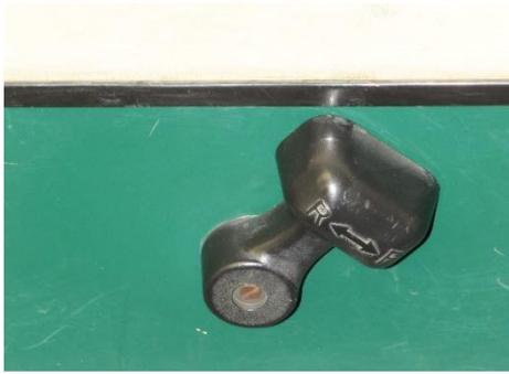
“reverse” or “neutral” before attempting to start. The “forward” position is towards the driver (F). The “reverse” position is towards the passenger (R) and in this position a warning sounder should operate.
