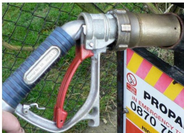
The gas release trigger at the end of the pipe may then be pulled open and clipped in the “open” position, using the little S (or Z) shaped clip at the back of the red trigger lever. There may be a brief noise of gas release as the trigger is pulled but this should stop and there should be no evidence of a gas leak once the pressures equalise.
