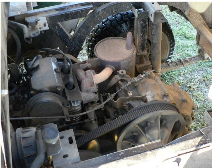
Check the condition of the main and starter drive belts.
