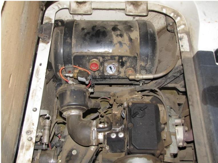
outlined for other vehicles and the winches in the following sections. The only way to determine the fuel level on these vehicles is to check the gauge on the gas cylinder (under the seat).
