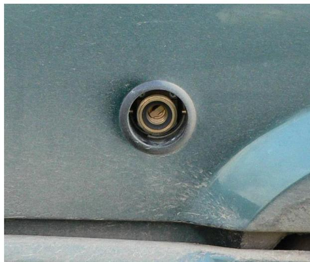
The Land Rover and other vehicles have external gas filling valves. The vehicle must be manoeuvred close to the gas compound, and the gas supply hose extended to the vehicle. On the end of the hose is a cylindrical fitting with a screw thread that should engage easily with the fitting on the vehicle and should be tightened by hand until no more movement is possible.
