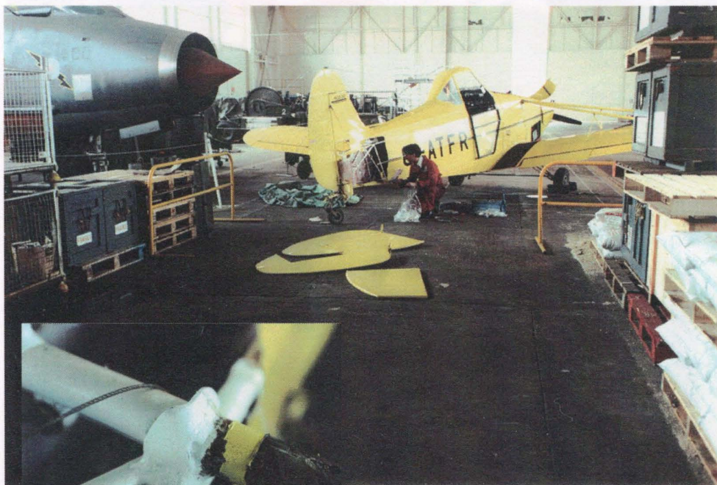
The Close-up shows the reason - metal fatigue.
